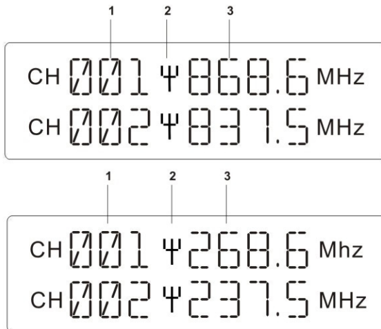
1.Channel display 2. Receive sign display 3. Frequency display
